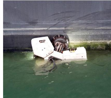
*Figure 1 The Fleet Cleaner robot cleaning a ship*
