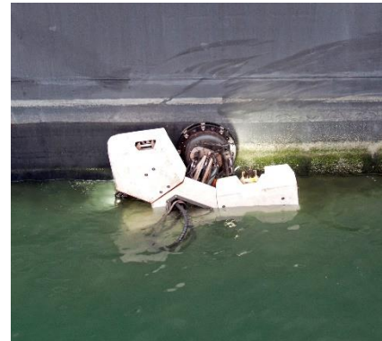
Figure 1 The Fleet Cleaner robot cleaning a ship
